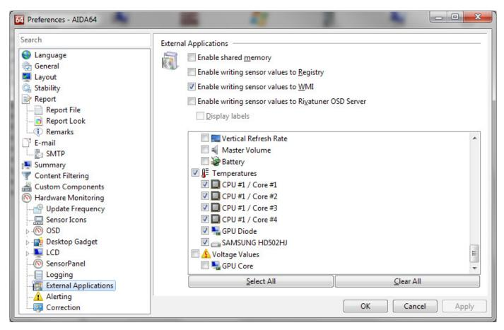
After activating "Use sensor with Aqua Computer Service" in the aquasuite, click the "Select data source" button to assign the currently selected software sensor to a temperature sensor provided by third party software.
