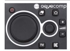
In "aquaero" mode, all keys will be processed by the aquaero and not forwarded to the PC. In "PC keyboard" and "PC media keys" mode, all keys will directly be forwarded to the PC and not be processed by the aquaero.
