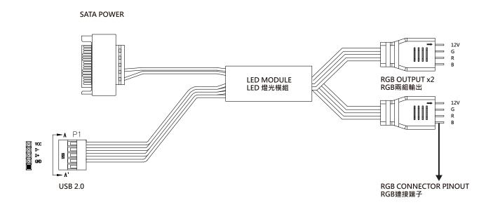
Note: If only one RGB output connector is used, please remove any additional RGB connectors in order to prevent a short circuit. 重要提醒: 若只使用一組RGB輸出端,請拔除另一組RGB連接端子,以防輸出短路。
