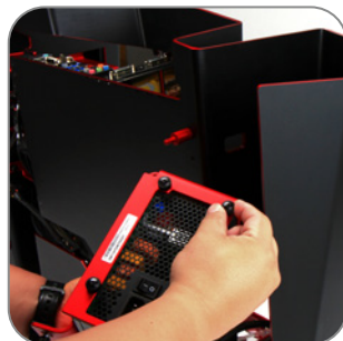
b. Install the power supply in proper location and secure it with screws
