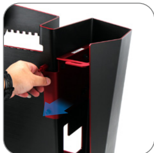
a. Loosen the thumb screws, and remove power supply bracket
