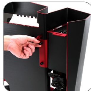
b. Install the power supply in proper location and secure it with screws
