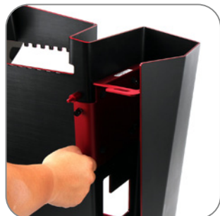
a. Loosen the thumb screws, and remove power supply bracket
