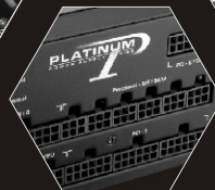
Full Modular Cabling
