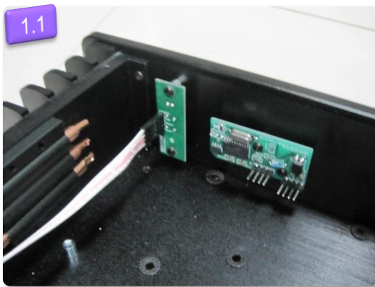
1.1 Installing IR receiver by accessories' screws, showed on page 10000.
