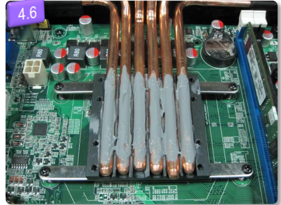
4.5 Wearing thermal grease on cooling panels' V bay.
