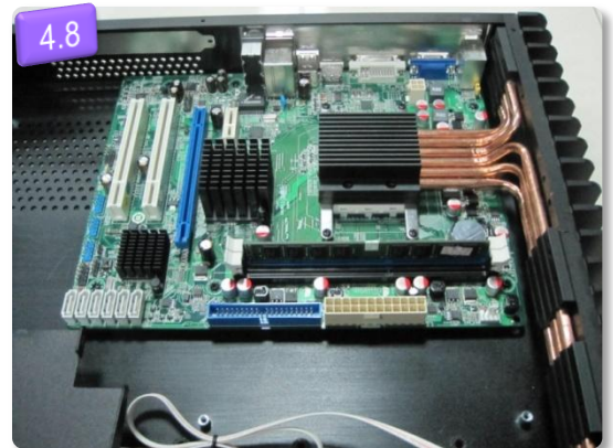
4.7 Coving motherboard cooling panels (up) (A) , Locking 4 screws (M)
