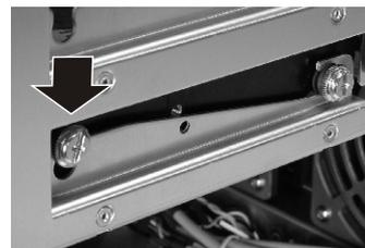
3. Press down the HDD into the slots to secure.
