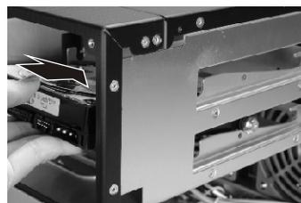
2. Slide the HDD into the HDD cage with the anti-vibration kit.
