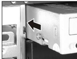
2. Slide in the drive into the slots as shown above.
