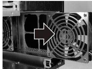
Fan mounted with tool-less anti-vibration kit, slide outwards to remove.
