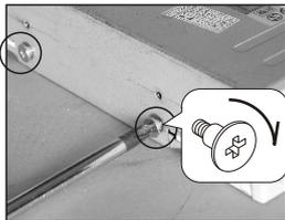
1. Secure screws on both sides for 5.25" drive.
