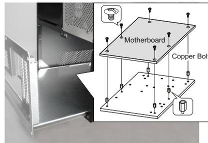
Secure the stand-off bolts on the M/B tray which match with the M/B fix points, place the M/B on the copper bolt, fasten the screws to secure.
