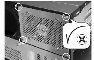
\* Remove 4 screws to remove the bracket.
