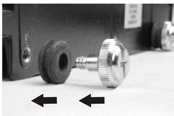
1. Fasten the HDD screws with anti-vibration rubber rings to the HDD.
