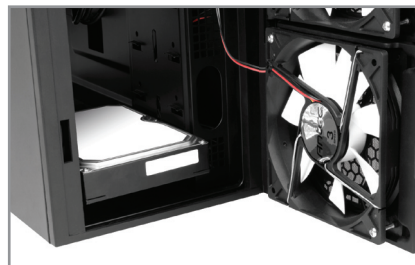
2 x internal 3.5" Fleet-Swap™ SATA bays (position changeable)
