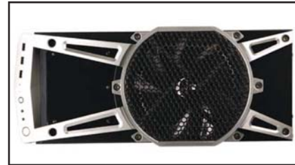
Massive cooling system highlighted by top 200 mm fan
