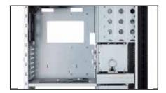
Divided upper and lower chamber structure the power supply resides in a separate chamber with dedicated cooling from a 120 mm fan to isolate heat from the system and lower system noise
