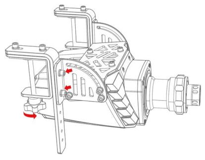
4. The height and rake angle are fully adjustable to accommodate different tabletop heights and driving preferences.
