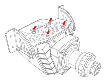
3. Attach the clamp brackets to the mount using 4 M6x12 screws with a spring washer and flat washer at a suitable height for your desk or profile rig. Fit the assembly to your rig or desk and fully clamp until secure using the star shaped clamp screw handles.
