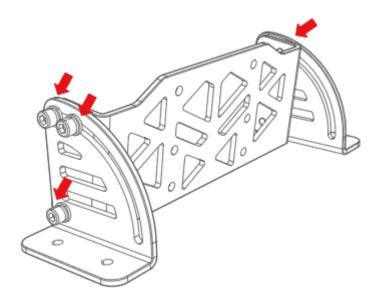
2. Attach the base to the mount using the supplied 4 x M6x12 screws and include a flat washer if needed for optimal tightening.
