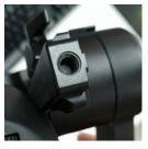
One 1/4 thread hole behind tilt motor.
