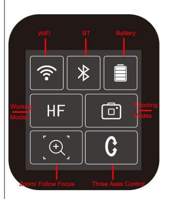
Screen Interfaces left touch controls: adjust the parameters of camera when wifi connection between gimbal and camera is done, including ISO, Exposure Compensation, Scenes, ect..
