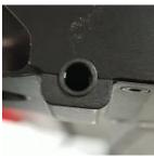
One 1/4 thread hole on the pan motor for installation of accessories.
