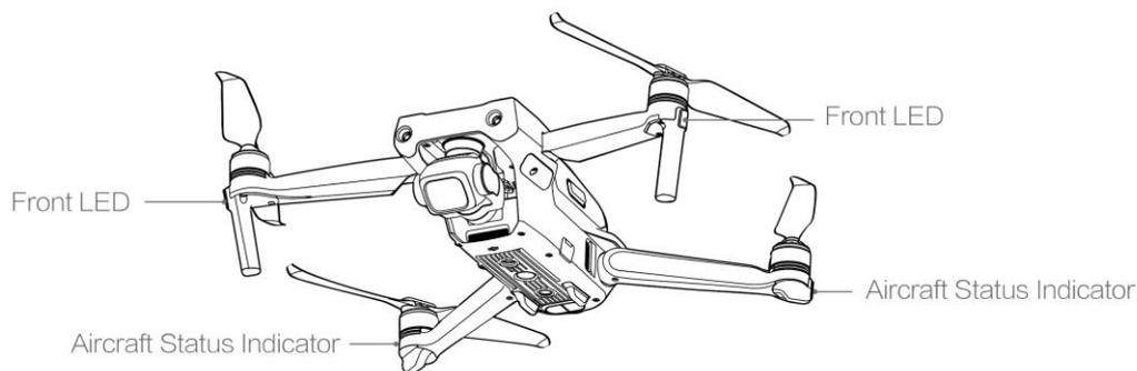
The front LEDs show the orientation of the aircraft and glow solid red when the aircraft is turned on to indicate the front of the aircraft.
