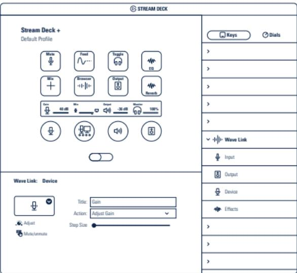
The Wave Link plugin allows you to customize your audio mixing controls and layout. Just drag and drop actions and effects onto keys and dials in the Stream Deck app. Configure your actions and interface icons exactly the way you want.
