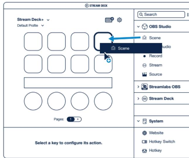
In the Stream Deck app, drag actions from the right panel and drop them onto your virtual Stream Deck + interface. You can add single or multiple actions to keys, dials, and the touch screen.
