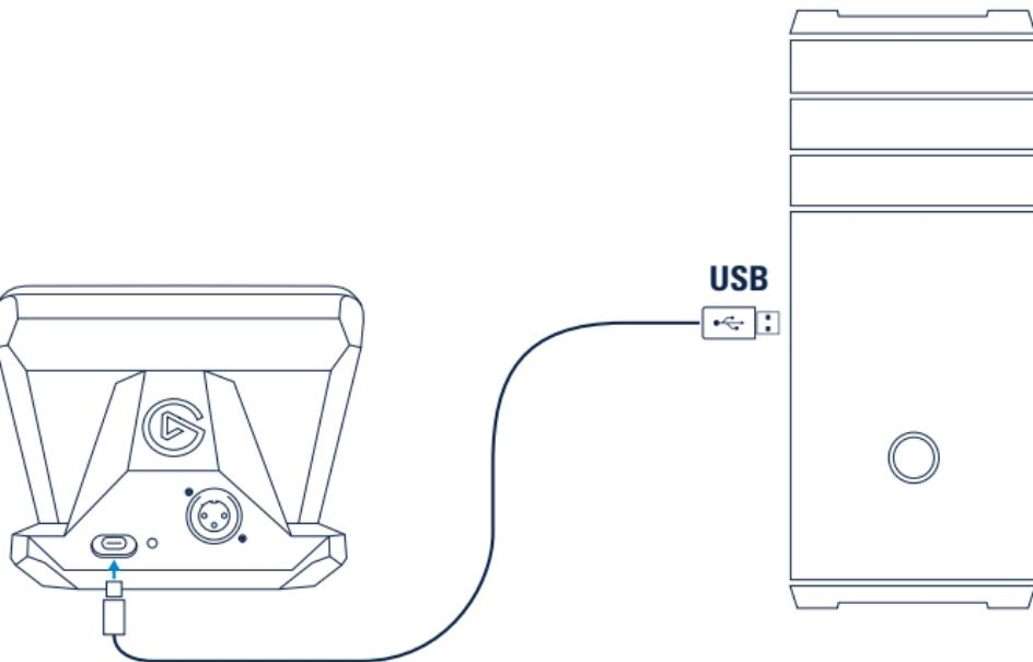
Connect the device directly to a USB port on your PC or Mac – do not use a USB hub.
