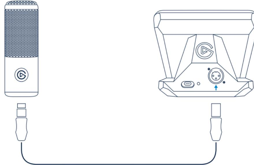
Connect your mic using a standard XLR microphone cable.
