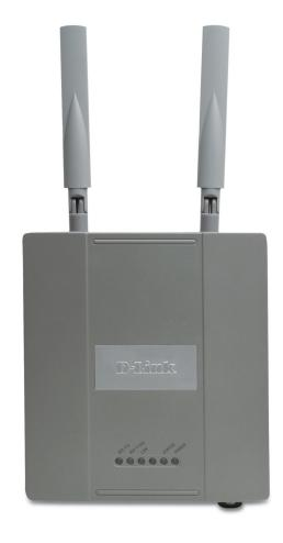
power to these locations is difficult and expensive. The DWL-8500AP can easily obtain power from a DWS-3024/3026 switch located as far as 100 meters away through the unused pairs of the existing network cable, doing away with the need to install separate power wiring. With industry-standard 802.3af PoE support, this wireless access point does not even require a PoE injector.
