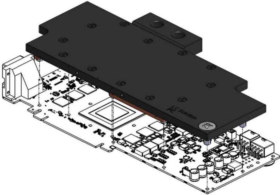
3. **ATTACHING BLOCK TO GRAPHIC CARD.** By using Philips screwdriver screw in enclosed M3x4 DIN7985 screws. EKWB recommends users to start tightening the screws around the GPU core and continue outwards. Always use a plastic washer under each and every screw!
