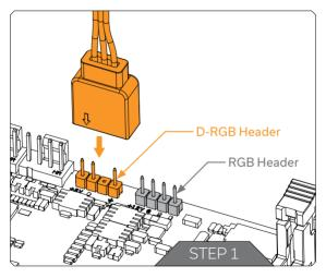
Plug the 3-pin connector from EK-Quantum Kinetic TBE D5 to the D-RGB header on the motherboard. The LED will work if the pin layout on the header is as follows: +5V GRB.
