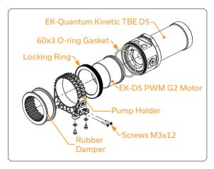
Install the EK-Quantum Kinetic TBE D5 onto the EK-D5 PWM G2 Motor. Make sure you install the provided 60x3 O-ring gasket. Reseat the gasket if needed. You can rotate the EK-D5 PWM G2 Motor if required.
