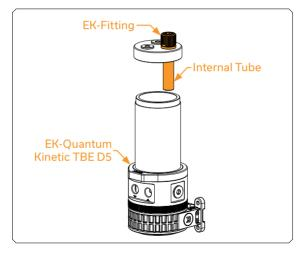
The internal tube, which is enclosed in a mounting kit, can be used for fluid intake into the reservoir. Make sure that the sealing gasket on the internal tube is placed correctly.
