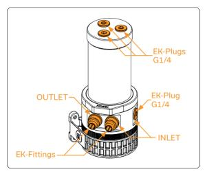
EKWB recommends using EK-Quantum Torque fittings with the EK-Quantum Kinetic TBE D5 PWM series reservoir pump combo units. If you use barbs ensure that the tubes are securely attached using hose clamps or an appropriate substitute.
