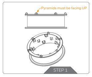
An alternative soft rubber damper is included. If excessive pump vibrations are transmitted through the mounting assembly then this can be used to reduce them further. When replacing the damper, take care that the pyramids face upwards as shown. Use of the soft damper is only recommended when the unit is installed vertically.
