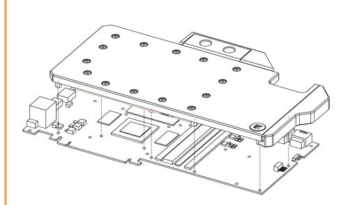
2. ATTACHING THE BLOCK TO THE GRAPHIC CARD. Use a Philips screwdriver screw with the enclosed M2,5x4 AX1 (15) screws. EKWB recommends users to start tightening the screws around the GPU core and continue outwards. <u>Always use</u> a plastic washer under each and every screw! If the washer is already present on the circuit board (usually around the four GPU core screw holes) there is no need for additional washer.
