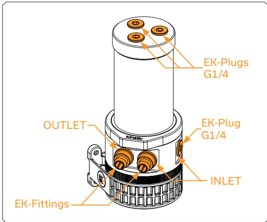
EKWB recommends using EK-Quantum Torque fittings with the EK-Quantum Kinetic TBE D5 PWM series reservoir pump combo units. If you use barbs ensure that the tubes are securely attached using hose clamps or an appropriate substitute.
