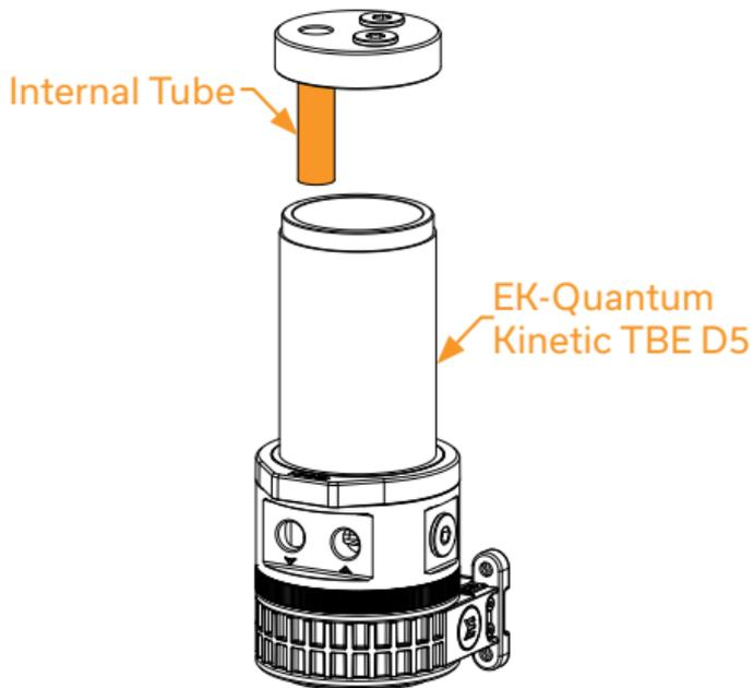
The internal tube, which is already pre-installed with the EK-Quantum Kinetic TBE D5 PWM, can be used for fluid intake in the reservoir.
