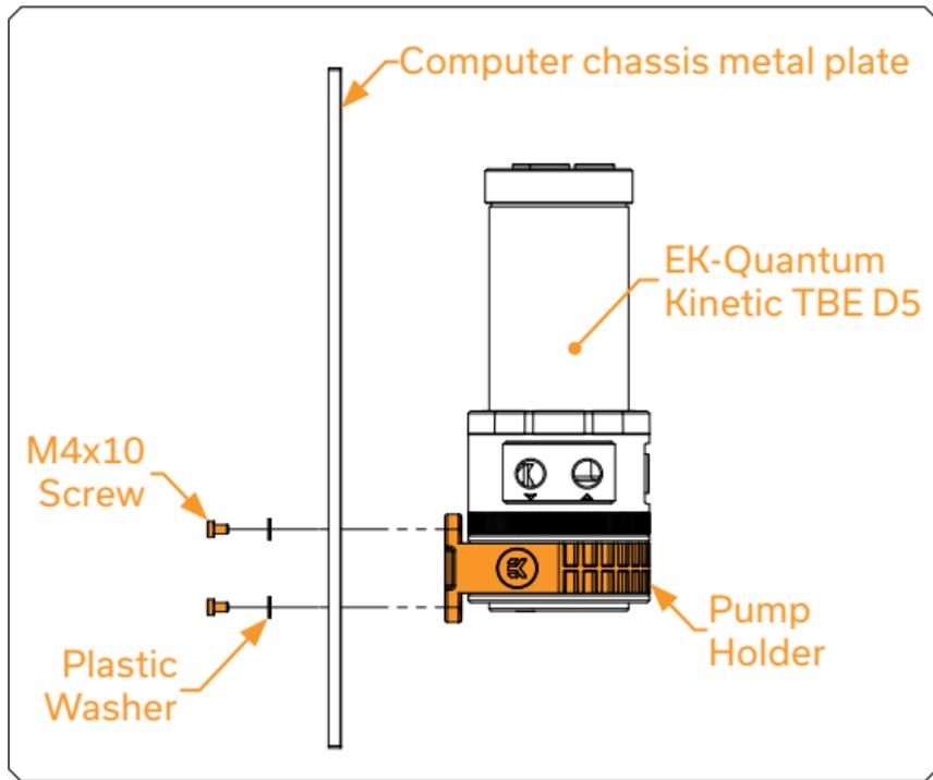
By default the EK-Quantum Kinetic TBE D5 ships with a pump holder that can be installed directly to the computer chassis. If there are no appropriate mounting holes available: user may need to drill 4 (four)  $\Phi 5$  mm holes through the metal chassis using an electric power drill. Included is a sticker which can be used to mark the hole centers accurately.
