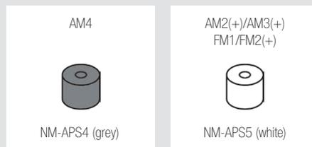
Use the grey NM-APS4 spacers for AM4 and the white NM-APS5 spacers for AM2(+)/AM3(+)/FM1/FM2(+).
