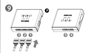
Connect the plug into the port in numerical order, start with plug one.
