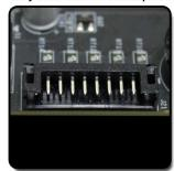
**ONBOARD CPU TEMP MONITOR**
